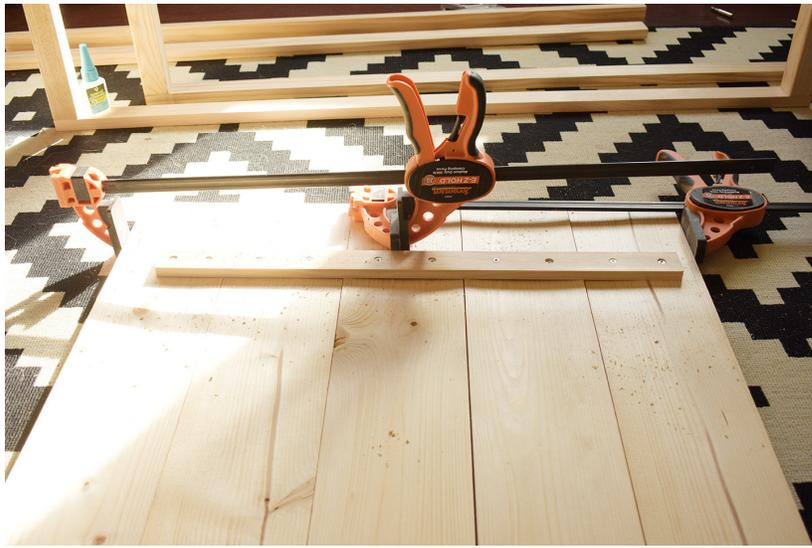
Clamp all five of the 4" x 48" boards together. If you don't have clamps that are long enough, you can hook two clamps together, as shown. Make sure you clamp your boards together with the edges lining up so your table isn't crooked.
