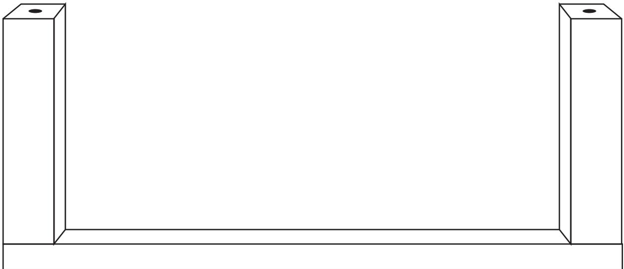
Once the RapidFuse is dry, pre-drill a hole through the 48" board into the Parson's leg. This step is important because the Parson's legs we used are made out of Walnut, which is a very hard wood that is difficult to screw in to. Use a 1 1/4" screw to help hold the legs to the board.
