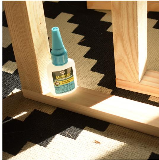
Once the screws are removed from all four legs, use Rapid-Fuse to adhere a leg to each end of two 1/2" x 2" x 48" boards. See illustration below. **IMPORTANT:** Make sure you glue the end of your leg that does NOT have the hole where you removed the screw. You need to glue the bottom of the leg that is flat, to the board.
