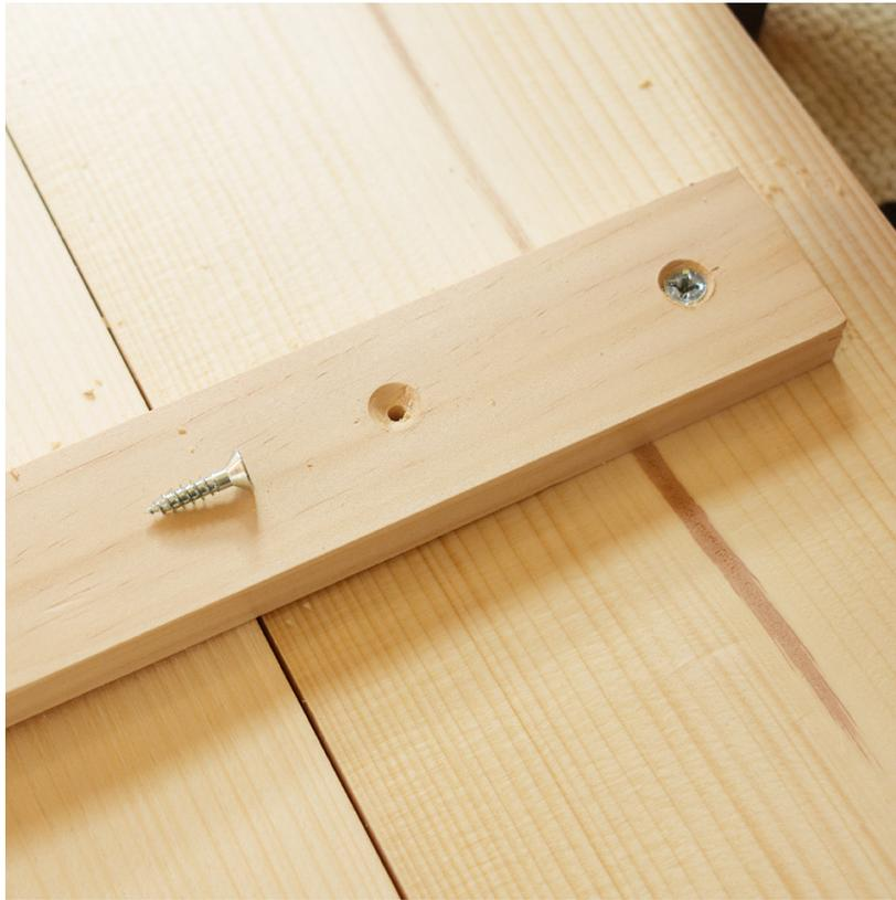
Apply RapidFuse to the back of a 1/2" x 2" x 24" board and lay it across the 48" boards. Use your drill and countersink drill bit to pre-drill holes through both boards. This step is important to keep your boards from cracking when you drill the screws in. Once your holes are pre-drilled, use a 5/8" screw to attach the 24" bracer board to each of the 48" boards with two screws per board.
